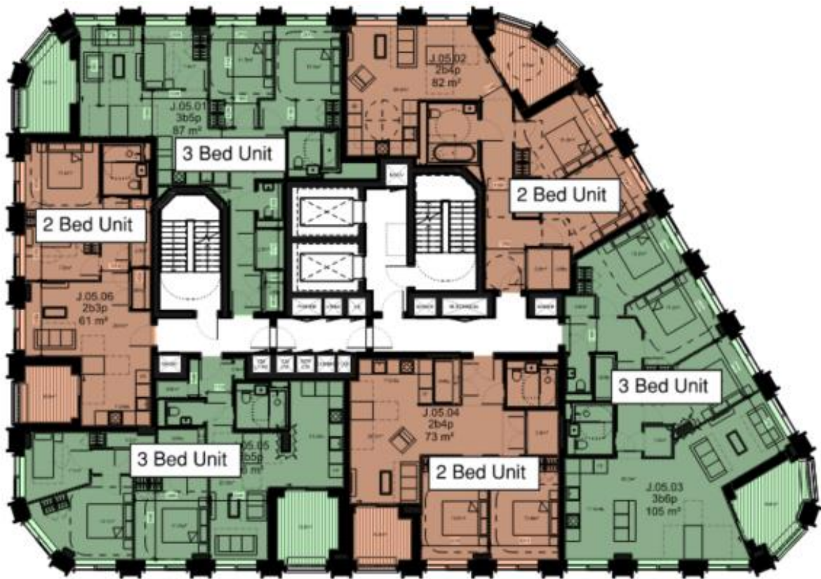
Figure 3: Block J - Typical Dwelling Unit Layout
